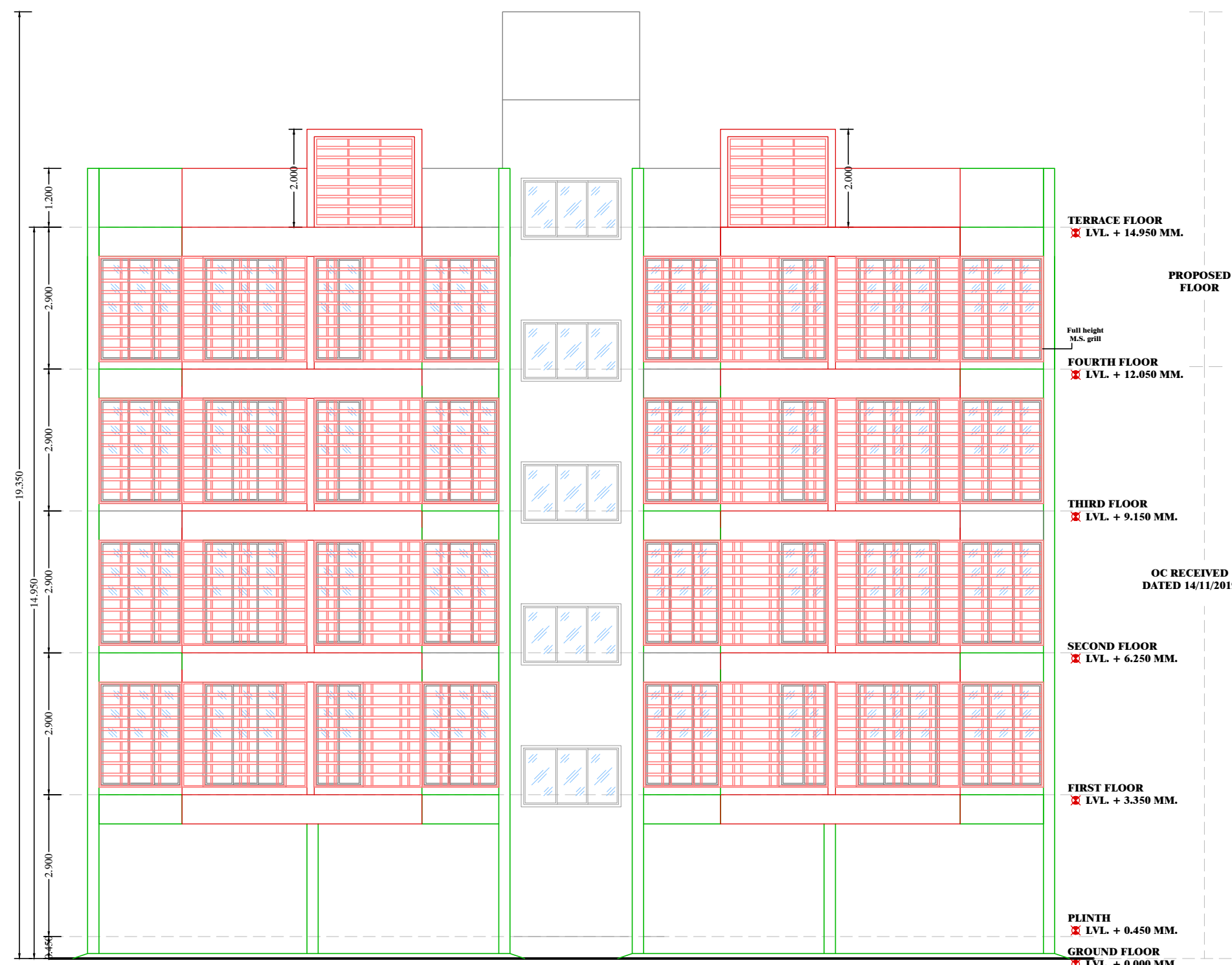
ELEVATION A (SCALE 1:100) BLDG. NO. 4
