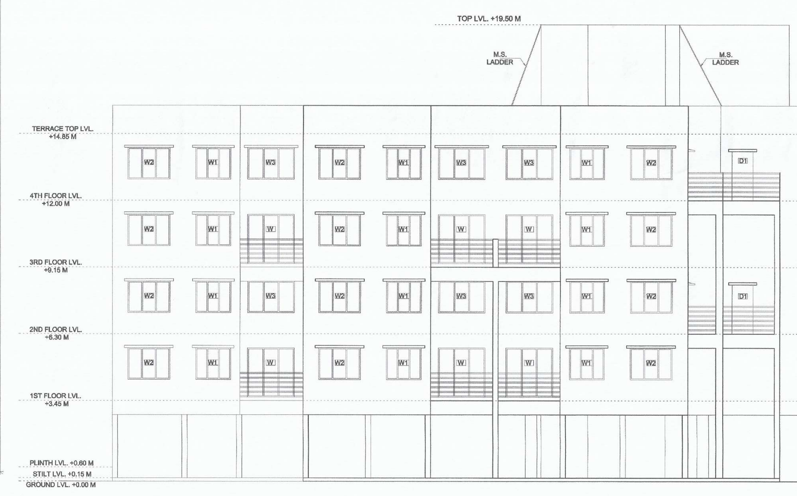
ROAD SIDE ELEVATION SCALE : 1:100
