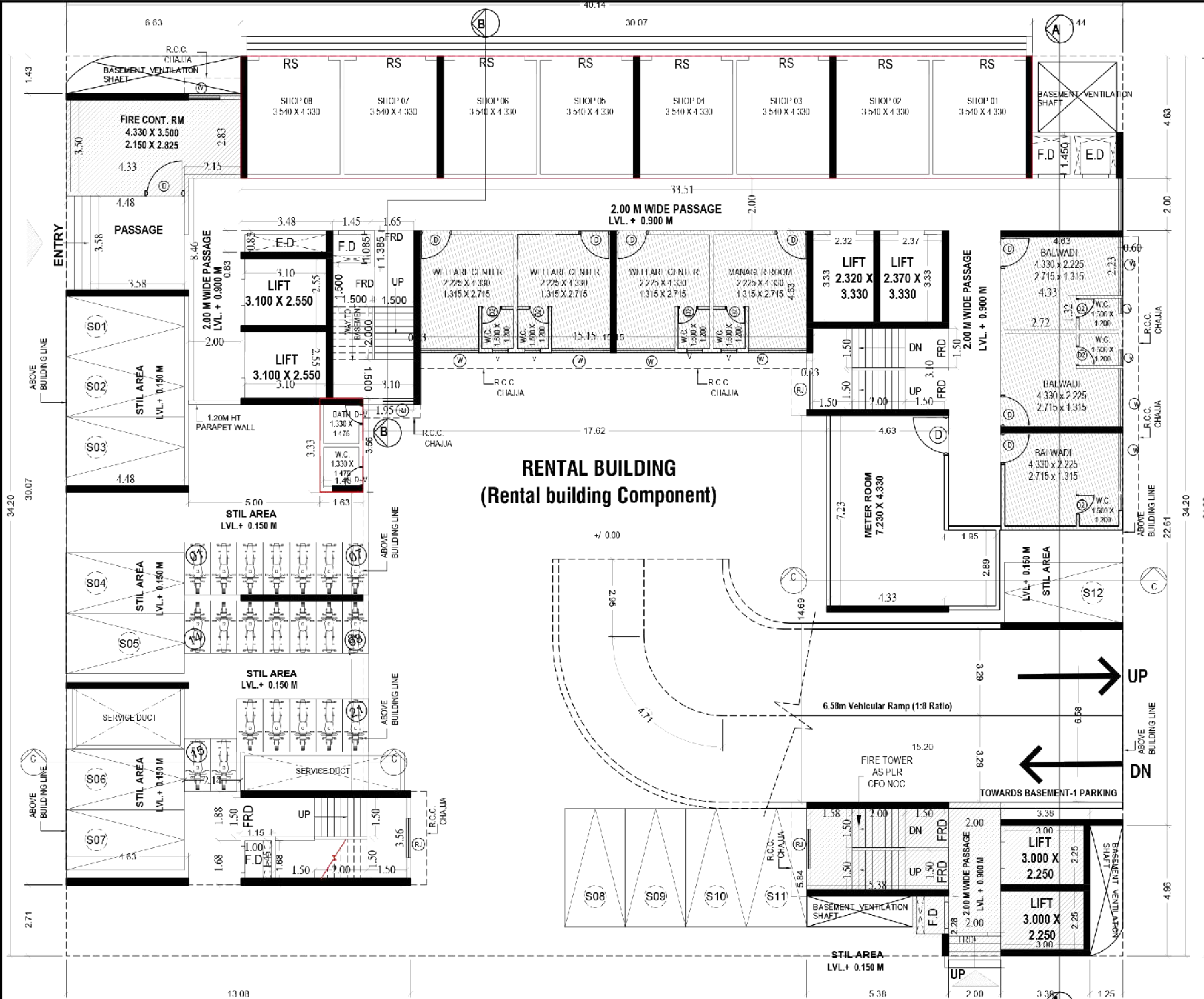
RENTAL BUILDING GROUND FLOOR SCALE :- 1:100
