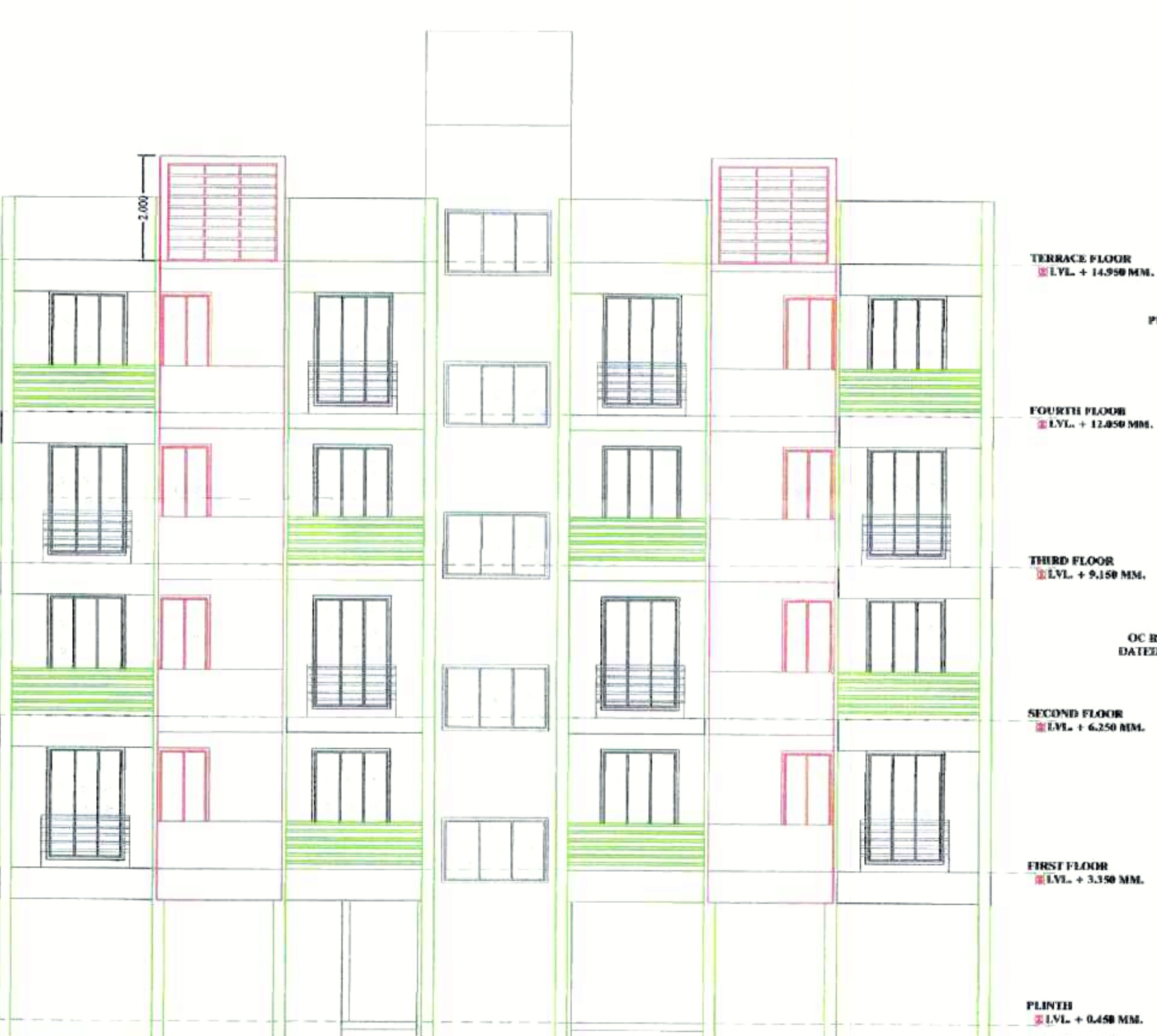
ELEVATION A BLDG. NO. 1 (SCALE 1:100)
