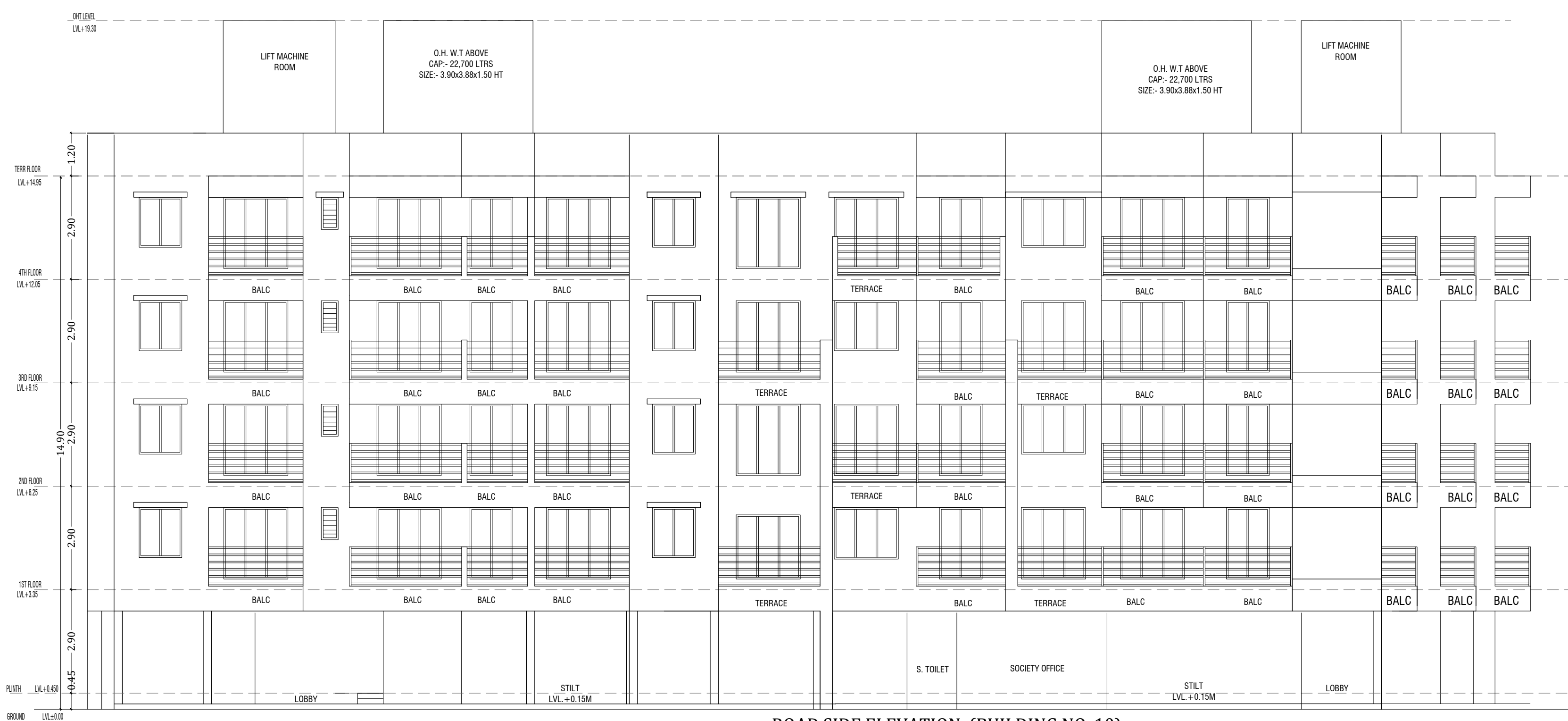
ROAD SIDE ELEVATION (BUILDING NO. 10) SCALE - 1:100
