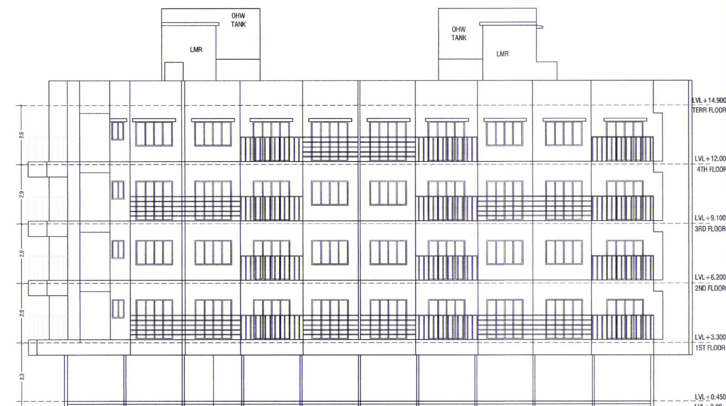
FRONT ELEVATION (WING-A & D) BLDG. NO.1 SCALE:1:100
