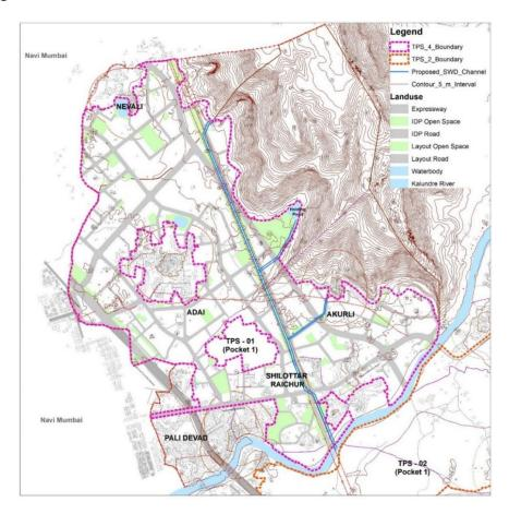
Figure 2 Proposed Storm Water Channel
